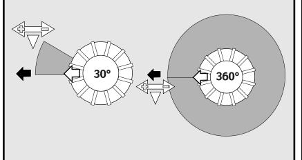
Turn the arc adjustment ring to align the white arrow to the right side of the watering arc.
